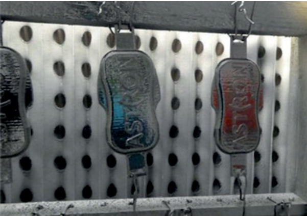
Figure 5: coated plastic parts with LDS lacquer
