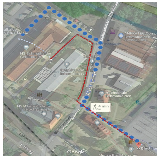
Fig. 5. Points derived from Google Maps (Blue) compared to Waypoints obtained through ANavS GNSS (Yellow)
