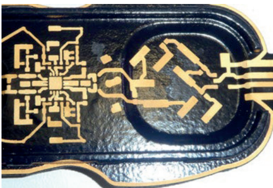
Figure 7: Conductors on a 3D MID component
